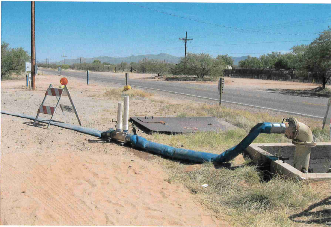
De Chlorinator used with 3" Ascorbic Acid Tablets Image from David Marquez , Tucson Water.
