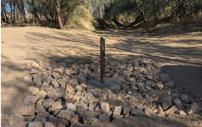
Flow metering device to measure the rate of stormwater flow into the Rita Ranch Detention Basin Project.
