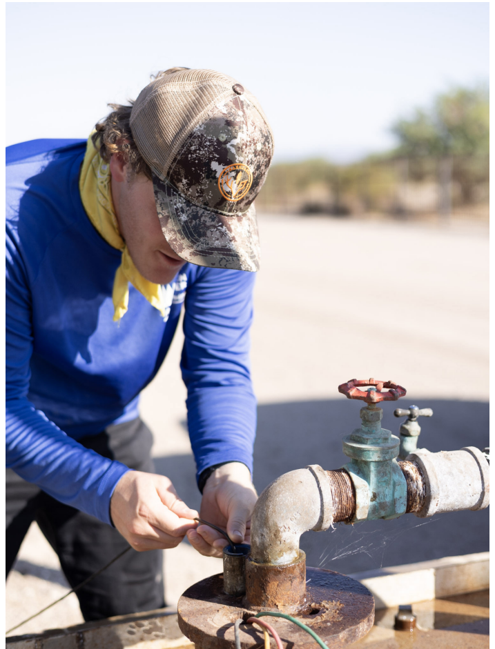
TW staff performing groundwater well measurement.
